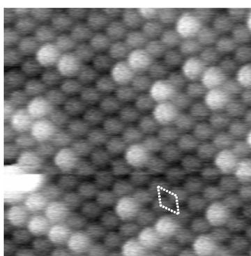
**Figure** Noncontact AFM image of Si(111) $\sqrt{3}\times\sqrt{3}$ -B surface. The brighter and darker spots correspond to Si-T<sub>4</sub> and B-S<sub>5</sub> structures, respectively. Scan size is 7.7 nm×7.7 nm.
