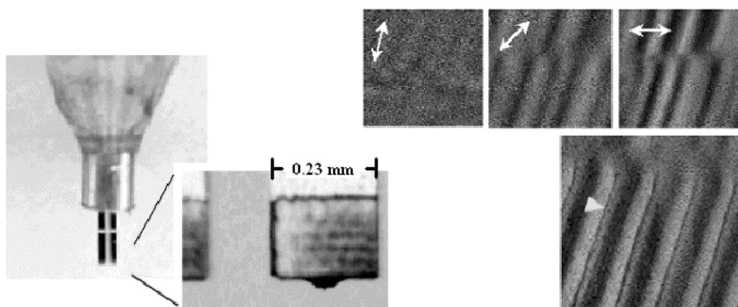
Figure 1. Optical microscope images of the tuning fork where a commercial MFM cantilever tip is glued to the bottom end of one prong.(left) Right top three shear-mode MFM images show the lateral variation of the magnetic force gradient. Arrows represent the dithering directions of the tip. And, the FWHM of the sharp line at the right bottom image is about 100 nm. Image dimensions here are 6  $\times$  6  $\mu$ m.
