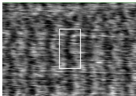
**Figure 1** Sub-nanometer resolution AFM image of ionic crystal  $\text{BaSO}_4(210)$  surface measured in water. Scan size is  $8\text{ nm}\times 5.6\text{ nm}$ . Rectangle is unit cell.
