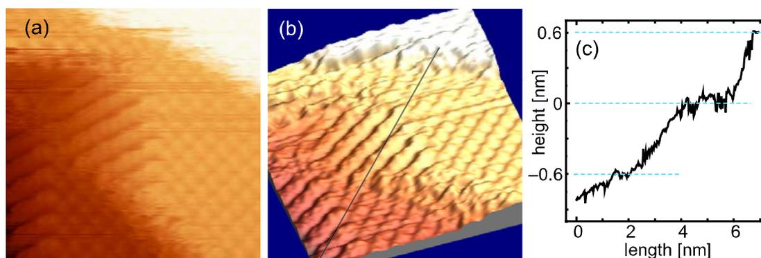
Fig.1. The atomic step structure formed by nanoscratching (a) the 2D topographic image of the  $\text{KCl}_{0.9}\text{I}_{0.1}$  cleavage surface ( $\Delta f = -18.6\text{ Hz}$ ,  $A_0 = 1.4\text{ nm}$ , scan size  $6 \times 6\text{ nm}^2$ ), (b) the 3D image of (a), (c) the line profile of (b) along the diagonal line in a black color
