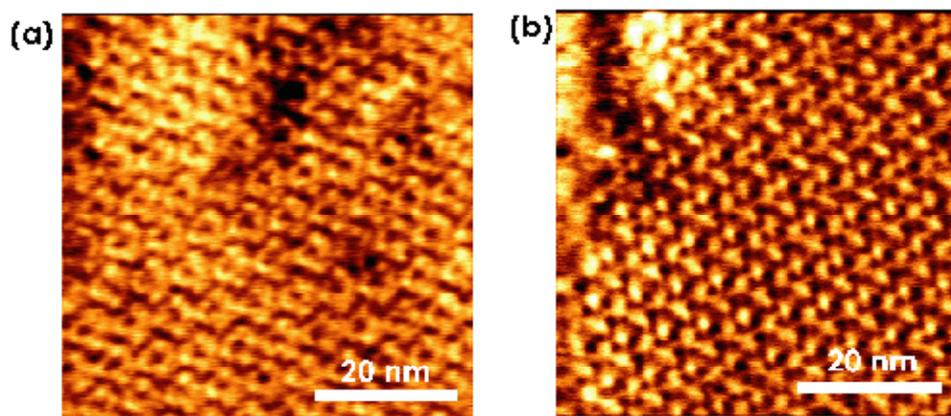
Figure 1 FM-AFM images of purple membrane in 150 mM KCl and 10 mM phosphate buffer solution (image size: 80 x 80 nm). Constant frequency shift image (a) ( $\Delta f = +205$  Hz, Amplitude = 4.5 nm) and constant height image (b) ( $\Delta f = +174$  Hz, Amp. = 3.7 nm) of the cytoplasmic purple membrane surface.
