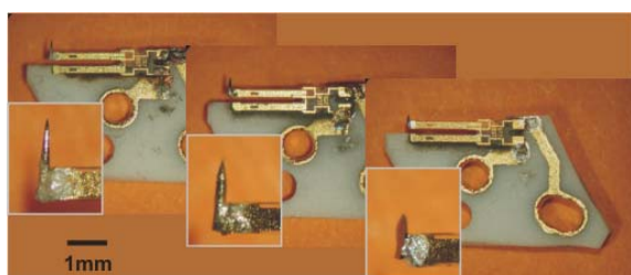
a) Sensors with W-, Co- and NiO-tip; Insets: tips magnified \sim 4x
